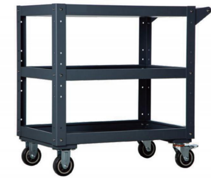
ITEM NO 719706 CART SIZE 750x500x800 900x500x800 1000x600x800 BOARD THICKNESS 1.5mm COLUMN THICKNESS 2.5mm
